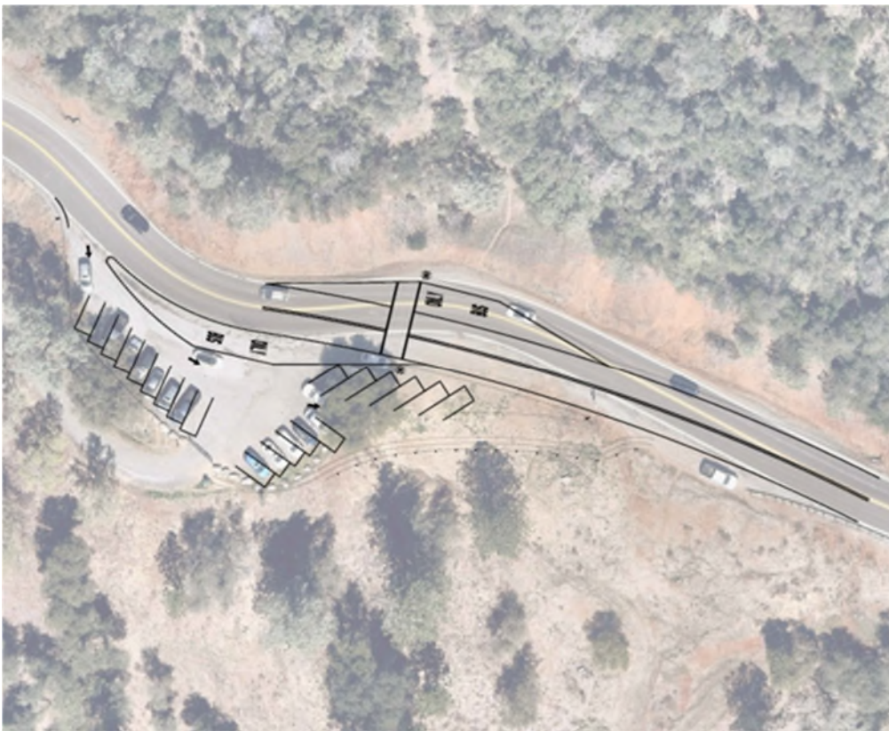
FIGURE 5959: CONCEPTUAL DESIGN FOR SHUTTLE STOP AT ROBIE POINT
