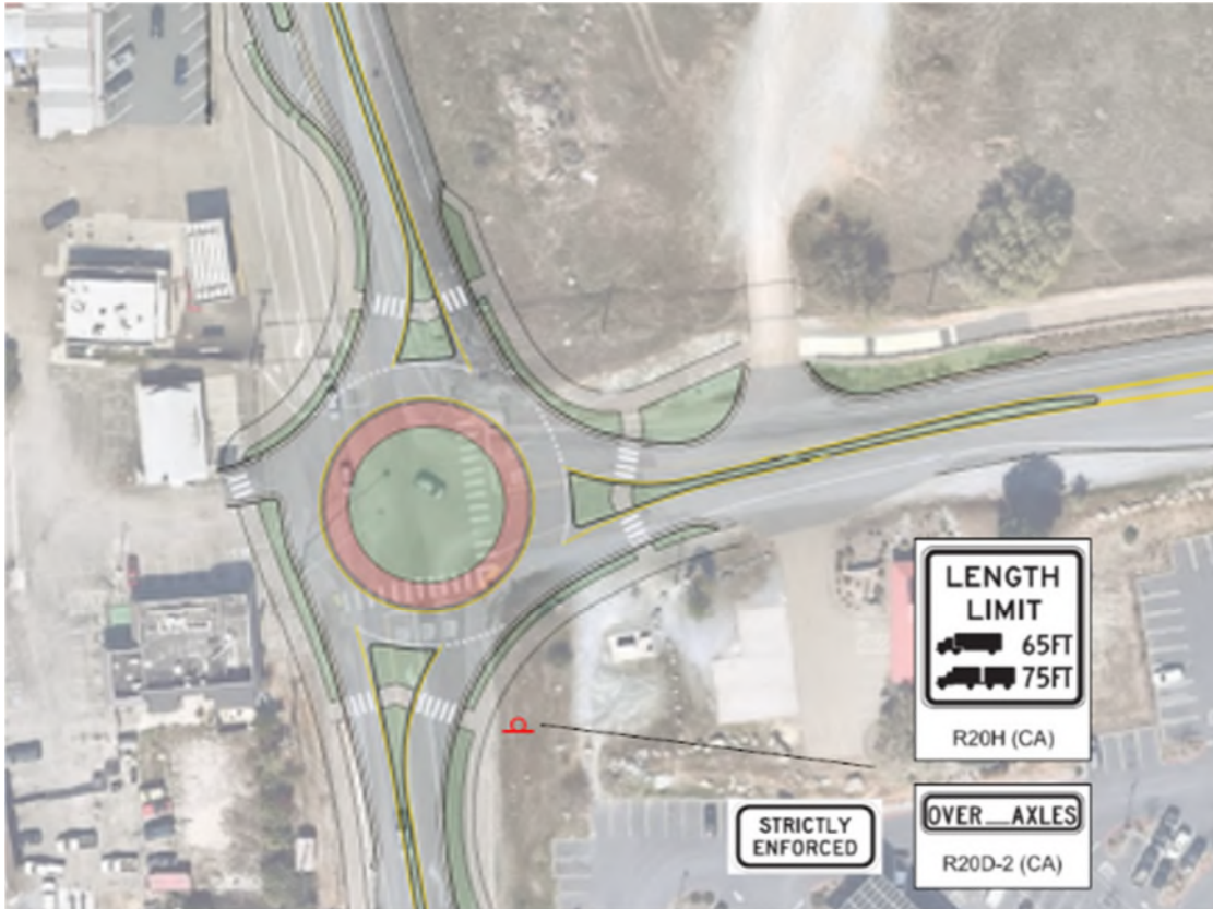
FIGURE 5757: CONCEPTUAL DESIGN FOR SR 49/SR 193 ROUNDABOUT
