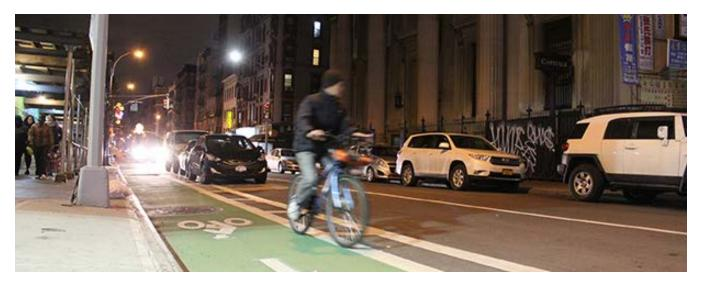
Protected Bikeways can be separated from the street with parking, planters, bollards, or other design elements.
